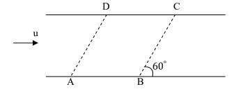
A river having parallel straight shores and width 3a flows with uniform velocity u. A, B, C, D are the vertices of the rhombus on shores as shown in the figure. Two persons P, Q who can swim with a speed  $v(v \ge u)$  with relative to water, start to swim from A at same time. P wants to swim from A to C and Q wants to swim from A to D. Using relative velocity theory, Draw the velocity triangles for the motion of P, Q on the same diagram.
