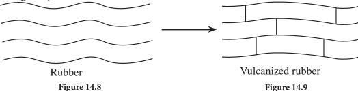
Vulcanized rubber is used to make tyres, tubes and battery cases.
