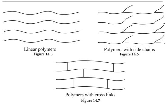
Have you heard about vulcanized rubber? Because of the elastic property of rubber, it is difficult to be used in some applications. By vulcanization, rubber can be made harder while decreasing its elasticity. During vulcanization natural rubber is reacted with sulphur. Then, cross links are formed among the linear chains of rubber through sulphur.
