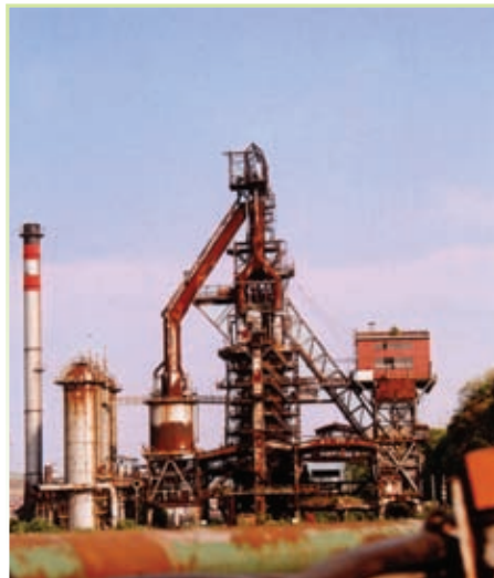
Figure 5.3 A furnace that smelts iron-ore
