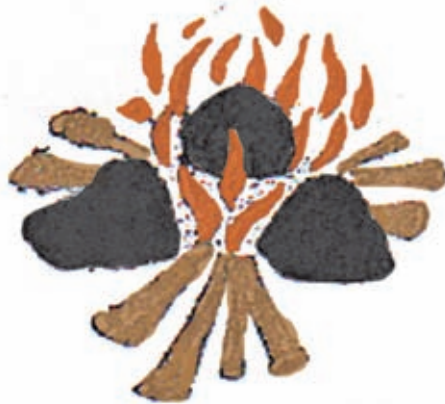
Figure 15.1- Carter's fireplace three-stone fireplace
