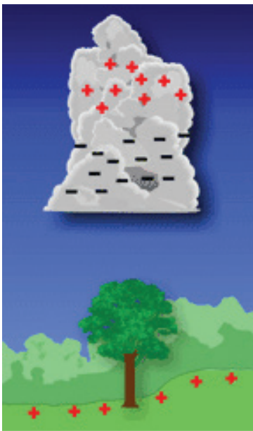
Figure 17.5 - Induction of positive charges on ground due to negative charges in the cloud
