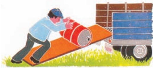
Figure 15.3 – Loading a barrel of oil to a lorry using an inclined plane
