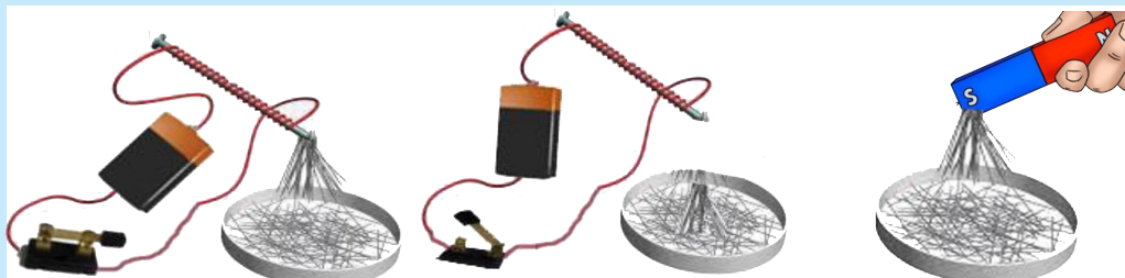
Figure 6.26 ▲ File clips fall off (do not attract) when electrical supply is disconnected
