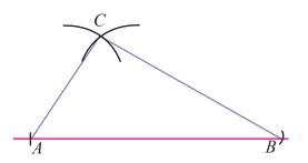
**Step 5** - After completing the triangle *ABC* by drawing the straight line segments *AC* and *BC*, measure the magnitudes of the interior angles by using the protractor, and write them down.
