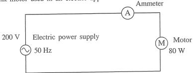
When the electric power supply was 200 V, the ammeter reading was seen as 0.5 A. Assume that the power loss in the ammeter is zero.
