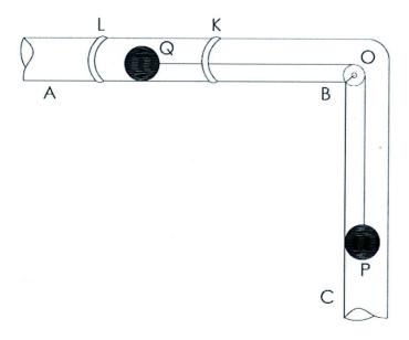
Shown in the figure is a smooth tube ABC of mass M, Right angled at B The tube passes through two smooth rings K and L. There is a smooth pulley O fixed at B. There are two particles P and Q with mass of each m at the two ends of an inelastic string that passes through the pulley. Find the acceleration of the particles due to the moment, relative to the tube, when the system is released freely.
