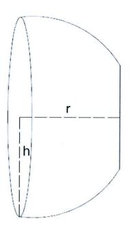
The figure shows a solid taken out from a uniform solid hemisphere of radius r using a plane parallel to the plane surface, perpendicular to the to the axis of symmetry and at a distance h from the center of the plane surface  $h(\leq r)$  Find the center of gravity of the solid using integration.
