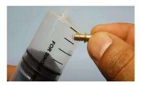
2) Fix the other value to the place where the needle of syringe is fixed. Be careful to fix the values in the correct direction. Use a piece of tube in order to fix the values properly.
