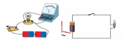
Activity 03 - Cut two pieces about 10cm long from the connecting wires. Connect the torch bulb using that. Now, keep the two batteries in series and connect the bulb. Then, observe the illumination of the bulb.
