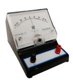
Galvanometer is used in the laboratory to identify the direction of current flow.
