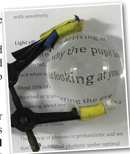
Figure 10.1 ▲ Letters are magnified when seen through a glass sphere
