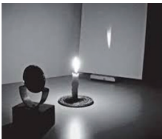
Figure 9.36 ▲ Instance of forming images from a concave mirror
