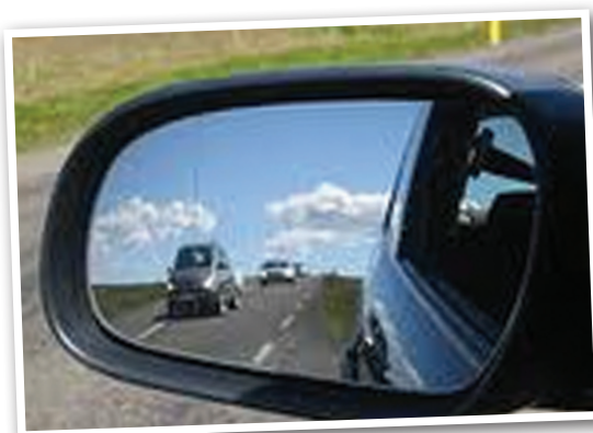
Figure 9.41 ▲ How rear side of a vehicle is viewed in a side mirror
