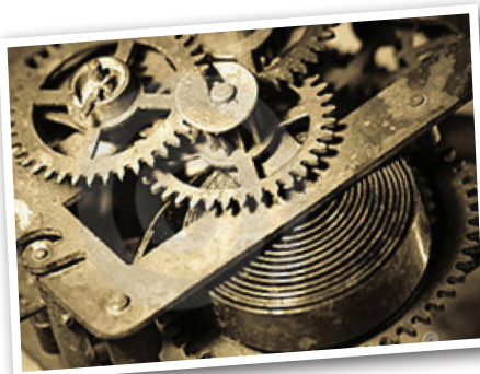
Figure ▲ 7.8 Inside a clock, that works by potential energy stored in a spring
