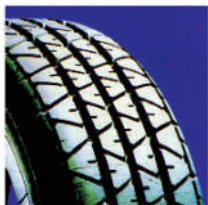
Fig. 6.14 - Grooves on tyres increases friction between the two surfaces
