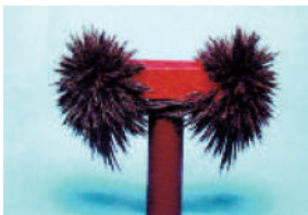
Fig. 6.22 - Poles of a magnet showing the attraction of iron powder
