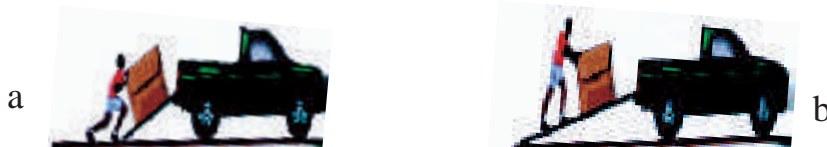
Fig 6.42 - a and b. How the work is made easier when the length of the inclined plane is more
