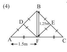
This is the figure of the cross section of the roof of a house supported by iron bars. In the triangle ABC, 'D', 'E' and 'F' are the midpoints of AB, BC and CA respectively. The length of EF is  $\frac{2}{3}$  of the length CA. ADF and FEC are C isosceles triangles. Considering the given information, find the total length of iron bars needed for this.
