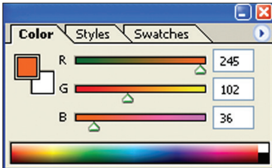
Figure 4.10 – The representation of RGB Triplet values for orange colour in Adobe Photoshop Colour Palette
