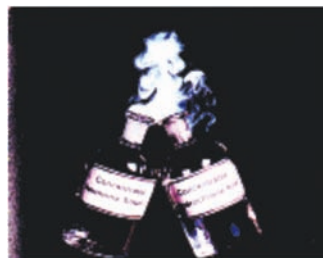
Fig. 3.13 Reaction of hydrochloric acid and ammonia
