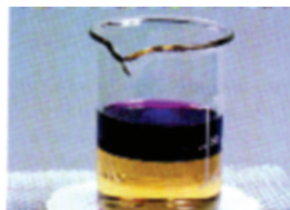
If you shake some cyclohexane with a solution of iodine in water, iodine goes into the cyclohexane layer.
