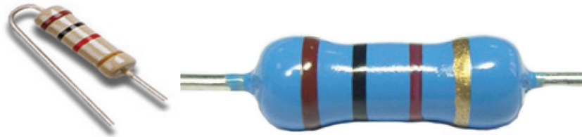
Figure 19.25 – Resistor values marked on the body of resistors using the color code method
