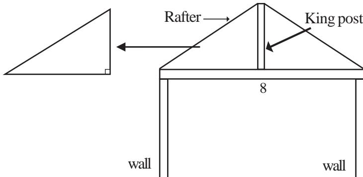
Consider a right angled triangle here. The distance from one end to the middle of the beam is 4 m. The length of the king post fixed at the middle, perpendicular to it is 1 m. The rafter makes the hypotenuse of the right angled triangle thus formed.
