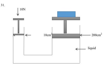
The diagram shows the energy transmission in a liquid. The area of A and B pistons respectively  $10 \text{ cm}^2$  and  $200 \text{ cm}^2$ .
