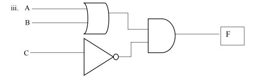
Write the Boolean expression of above circuit using A,B and C as inputs. (2 Marks)
