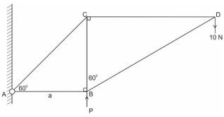
It is given that AB = a and  $C\hat{A}B = C\hat{B}D = 60^{\circ}$ . A weight of 10N is suspended from D and the frame work is hinged to a vertical wall at A. The framework is kept in equilibrium in a vertical plane by a vertical force applied at B, so that rods AB and CD are horizontal and the rod BC is vertical. Find the value of P.
