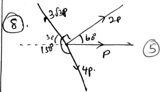
$$\begin{aligned}\vec{x} &= P + 2P \cos 60^\circ - 3\sqrt{3}P \cos 30^\circ + 4P \cos 60^\circ \quad (5) \\ &= P + P - \frac{9}{2}P + 2P \\ x &= 4P - \frac{9}{2}P = -\frac{1}{2}P\end{aligned}$$
