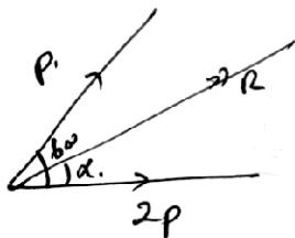
$$\begin{aligned} R^2 &= p^2 + (2p)^2 + 2(p)(2p) \cos(60^\circ) \quad (10) \\ &= p^2 + 4p^2 + 4p^2 \times \frac{1}{2} \\ R^2 &= 7p^2 \\ R &= \sqrt{7}p. \quad (5) \end{aligned}$$
