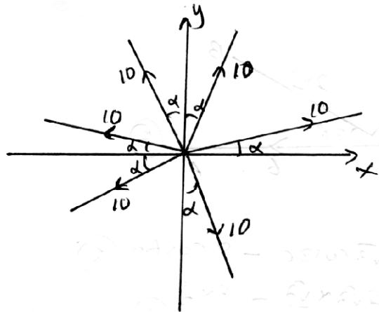
$$\begin{aligned} \rightarrow x &= 10 \cos \alpha + 10 \sin \alpha - 10 \sin \alpha - 10 \cos \alpha - 10 \cos \alpha + 10 \sin \alpha \\ &= 10 \sin \alpha - 10 \cos \alpha. \\ &= 10 (\sin \alpha - \cos \alpha) \quad (5) \end{aligned}$$
