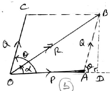
$$\begin{aligned} OB^2 &= OD^2 + BD^2 \\ P^2 &= (P+Q \cos \alpha)^2 + (Q \sin \alpha)^2 \\ P^2 &= p^2 + Q^2 + 2pQ \cos \alpha. \quad (10) \end{aligned}$$
