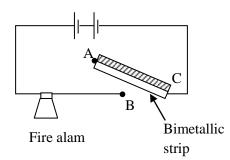
c) The bimetallic strip indicated by AC in the above figure is made by riveting a strip of iron and a strip of brass together.
