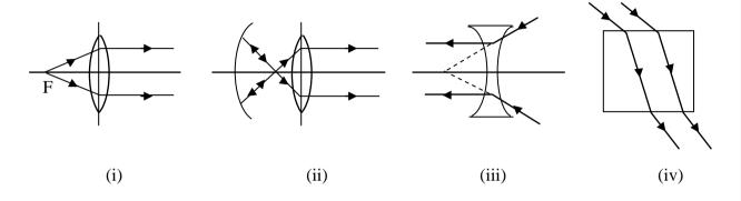
2) The critical angle for two media A and B is 35°. Where A is optically rare and B is optically denser. Which of the following correctly illustrate the path of a light ray. (Angle of incidence is 42°)
