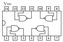
When the input values of 0, 1, 1, 1, 1, 0, 0, 0 to the pins. 1, 2, 5, 6, 8, 9, 12, 13 respectively are given, what are the output values for the pins 3, 4, 10, 11 respectively.
