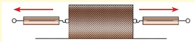
Figure 12.5 – Pulling a block of wood in two directions
