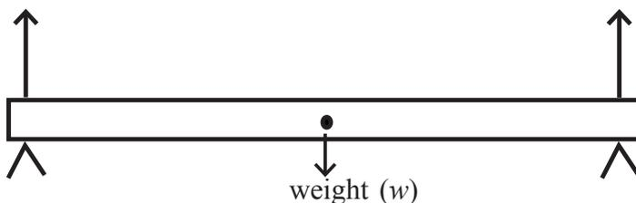
Figure 12.9 - A rod resting on two supports
