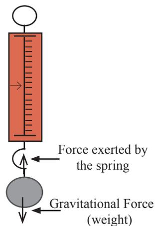
Figure 12.2 - An object suspended by a spring balance
