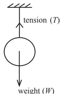
Figure 12.3 – A sphere suspended by a string
