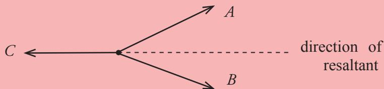
When the resultant of the two forces *A* and *B* is applied in the direction of the force *C*, the three forces will be in equilibrium.
