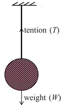
Figure 12.7 - An object suspended by a string
