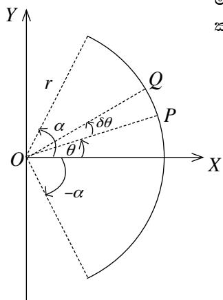
$$\begin{aligned}\bar{x} &= \frac{\int_{-\alpha}^{\alpha} mr^2 \cos d\theta}{\int_{-\alpha}^{\alpha} mr d\theta} \\ &= \frac{r [\sin \theta]_{-\alpha}^{\alpha}}{[\theta]_{-\alpha}^{\alpha}} \\ &= \frac{r \cdot 2 \sin \alpha}{2\alpha}\end{aligned}$$
