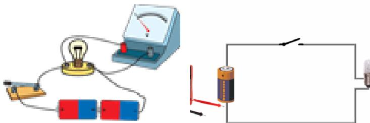
Activity 03 - Cut two pieces about 10cm long from the connecting wires. Connect the torch bulb using that. Now, keep the two batteries in series and connect the bulb. Then, observe the illumination of the bulb.
