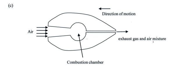
The diagram above is a rough diagram of an aeroplane jet engine. When the aeroplane moved in a speed of 250 m s<sup>-1</sup> the rate of air intake to one jet engine is 220 kg s<sup>-1</sup>. The fuel burn inside the combusion chamber exors gas and the air mixture exit with a speed of 420 m s<sup>-1</sup> from engine.
