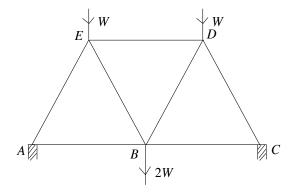
A framework made of seven light rods of equal length is shown in the diagram. It is kept on two supports at *A* and *C*, in equilibrium in a vertical plane, and the loads 2*W*, *W* and *W* are applied on the framework at *B*, *D* and *E* respectively.
