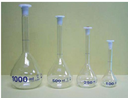
Volumetric flasks corresponding to the volume of the solution
