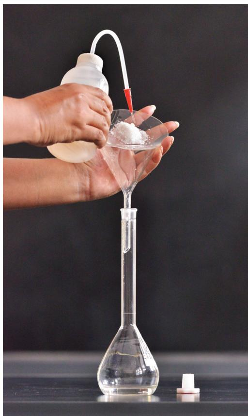
**Figure 3.2.2 - Preparation of a standard solution**
