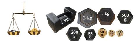
A balance scale (weighing scale) is used to measure the mass of an object by comparing it with the mass of one or more standard weights.
