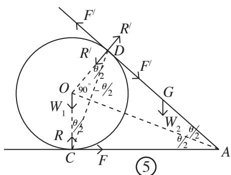
Since the weight of the cylinder and the force applied on the cylinder by the rough horizontal plane pass through the point  $C$ , the force applied on the cylinder at the point  $D$  by the rod should also pass through  $C$ . (5)
