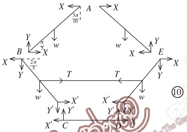
Let the length of a rod be  $2a$ . The system is symmetric about the vertical line through  $A$ .
